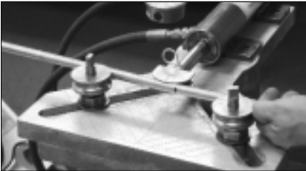
figure 6: Photo showing a tube in the bending process to show possible "droop"
