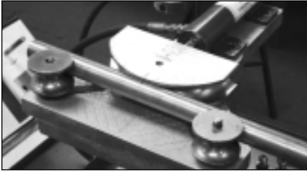
figure 2: Photo showing location of bend point
