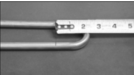
figure 7: Show 180° bend in progress
