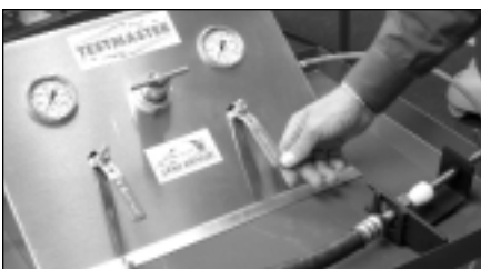
figure 6: Photo closing the dump valve.
