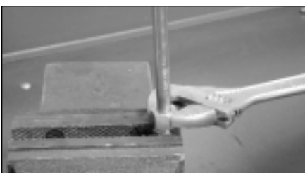
figure 18: Photo showing vise w/tech tightening nut
