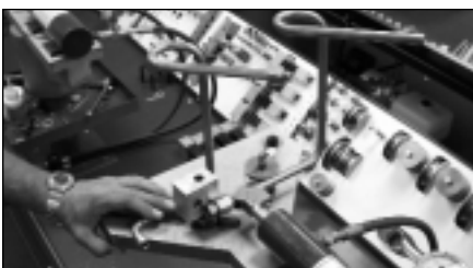
figure 13: Photo showing use of extreme close end bend die
