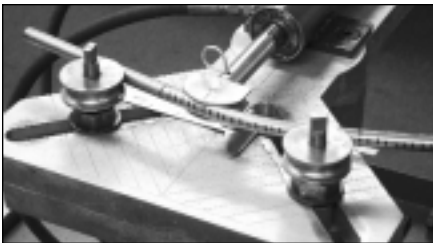
figure 6: Photo showing underbend and overbend tube in bender
