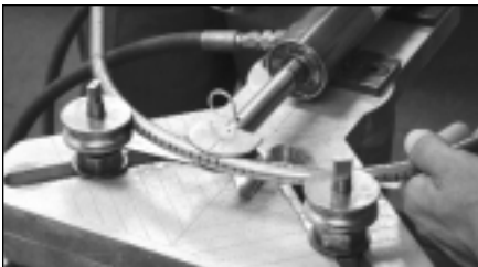
figure 6: Photo showing underbend and overbend tube in bender
